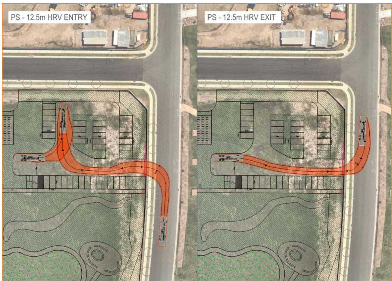
Figure 34: Swept Path of Proposed Loading Area
